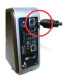
**Step 3.** Connect the square end of the USB cable to the hard drive. Then connect the flat end of the USB cable to the USB port on your computer.
